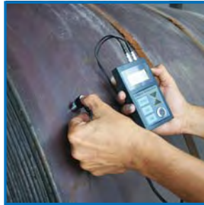
2. Ultrasonic Thickness Checking
