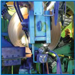
4. Spiral Pipe Forming
